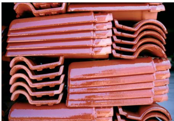
5. The weight of roofing tiles is limited (< 2.5 kg)
